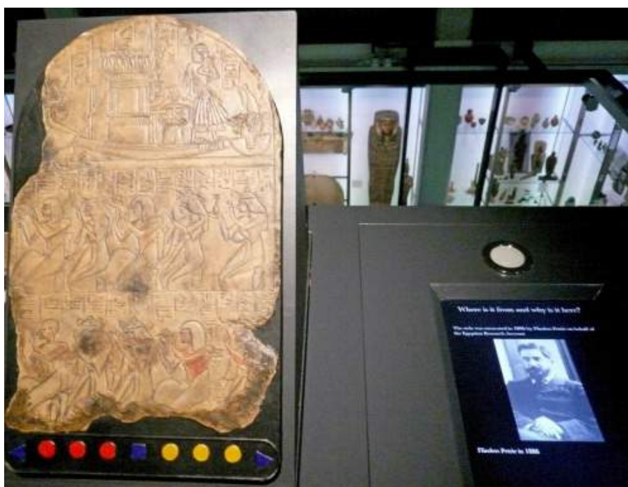
Fig. 5. Digital touch replica prototype of the Stela of Hesysunebef on Exploring objects gallery at Manchester Museum. When the replica is touched, information plays out on the adjacent screen as an image and an audio file.
